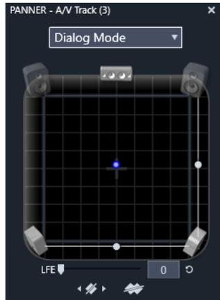
*Positioning the clip audio using the Panner in Dialog Mode. Note that the icons for the front corner speakers are translucent, indicating that they are not used in this mode. As adjusted here, the audio for the track will be heard coming from the right.*
