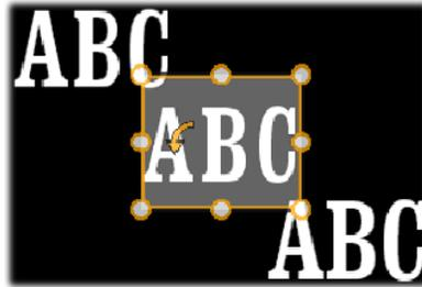
*In this example, a Look with three detail layers has been applied to a single text layer. The detail layers are configured identically except for their offset values, as follows: top left (-1.0, 1.0); center (0, 0); bottom right (1.0, -1.0).*
