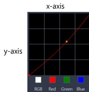
The x-axis of the graph represents the original tonal values (from highlights on the right, to shadows on the left); the y-axis of the graph represents the adjusted tonal values (from dark/less color at the bottom, to light/more color at the top).
