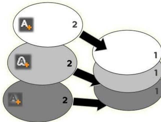
Face, Edge and Shadow: A new face detail (left, top) is added above the uppermost existing face layer; new edge and shadow details are added below the bottommost layer of their respective types.
