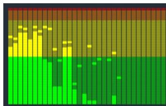
*The frequency spectrum breaks down the audio signals by frequency bands, showing the sound level in each band. Lower frequencies are on the left. Peak levels are shown as a small box above each main bar for which a peak has been detected in the past few seconds.*
