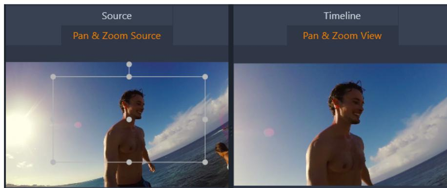
*In this illustration the Pan-and-zoom tab has been selected and remains set to the default Static mode. The selection frame, defines a region of the image that will be magnified to fill the entire frame, as shown on the right.*
