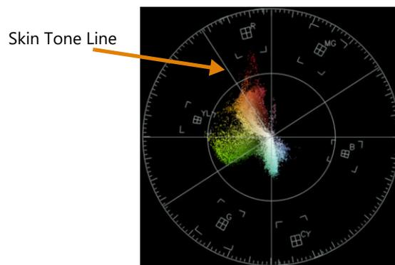
**Selective Vectorscope:** This feature is often used to identify and correct skin tone in a video. By using a brush to select skin tones in a video frame, you can use the vectorscope to ensure that the skin tones are aligned along the skin tone line.
