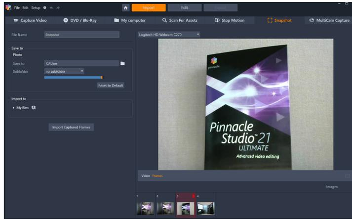
*Capturing snapshots in the Importer. While previewing live or taped video in the central area of the window, use the Capture Frame button to grab still images. Grabbed frames accumulate in the Image Tray at the bottom of the window until you click the Import Captured Frames button to transfer them to the Library.*
