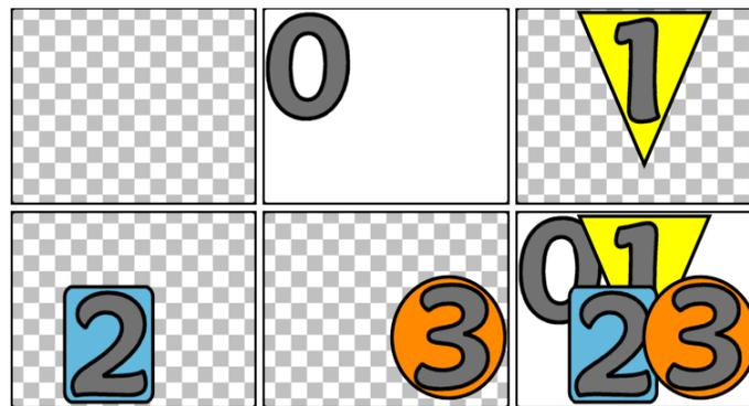
*Building up an image in layers starting with an empty frame (top left). The checkerboard pattern indicates transparency. Although backgrounds can have transparent or translucent areas, here we add an opaque background (0) for clarity, followed by successive layers with some opaque content (1, 2, 3). In the final composition (bottom right), upper layers obscure those below.*
